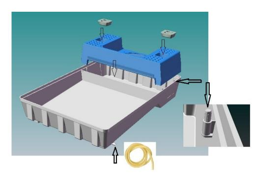
Make sure the 4 pins located on the Base are properly inserted in the Mist Generator (MG) housing.
